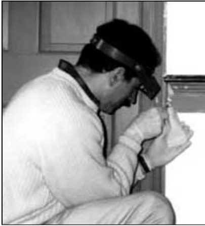
This conservator is shown collecting paint samples onsite. Then, in a laboratory, an ultra violet light microscope will be used to identify pigment and binding media. Photo: Courtesy, Matt Mosca.
