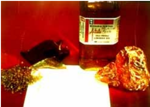
The basic ingredients (clockwise, from left) are chalk, glue, linseed oil, and resin. Photo: Jonathan Thornton.
