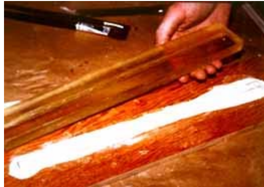
This finished length of compositum molding is stuck to its pressing board. The newly made piece will be sliced off the board, then applied. Photo: Jonathan Thornton.
