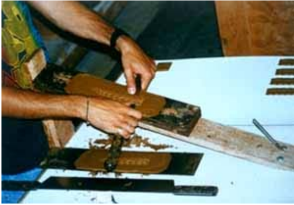
Ornament is being sliced from a pressing board. Photo: Lenna Tyler Kast.
