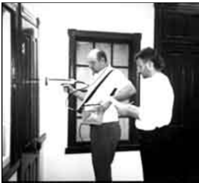
A licensed professional uses an x-ray fluorescence scanner to determine--without disturbing the surface--whether lead is present in underlying layers of paint. Photo: NPS files.
