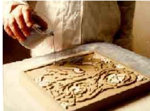
Colored slip, or liquid clay, is being poured into the indented portion of a reproduction encaustic tile, to create the pattern. Photo: H & R Johnson Tiles.
