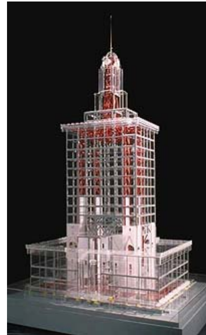
This computer model illustrates the comprehensive methods used to fully reinforce a building for the future. Oakland City Hall, CA. Computer Model ©Douglas Symes, San Francisco.
